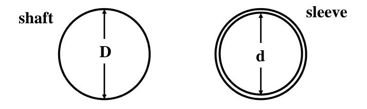
A cylindrical brass sleeve is to be shrunk-fitted over a brass shaft whose diameter is 3.212 cm at 0 °C. The diameter of the sleeve is 3.196 cm at 0 °C.
